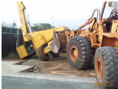
Front-end loader supports aerial lift
